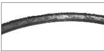
Shining surface due to high slippage
